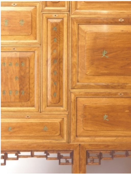
This photo shows details of the 18th century Chinese Dynasties Histories Case featured on the cover of this month's issue. The piece was done in butternut with an oil stain and lacquer. The case is a reproduction and is comprised of 15 boxes, each giving the history of a particular dynasty. The 59 carved characters are clerical Chinese. They were finished with copper patina paint to replicate the look of the original case.
