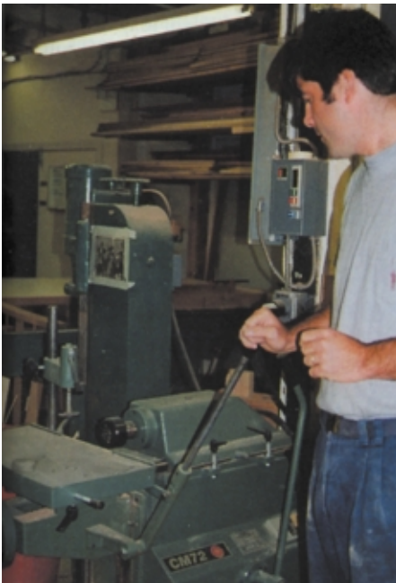
Englander's co-op shop houses a variety of woodworking equipment, including this Bini CM72 horizontal boring machine. Englander uses it for mortise and tenon joints.
